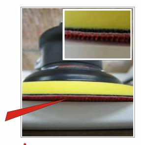
! Using SPECIAL PADS glue remainder will be taken away simply and easily - without damage to the surface of the parts.
