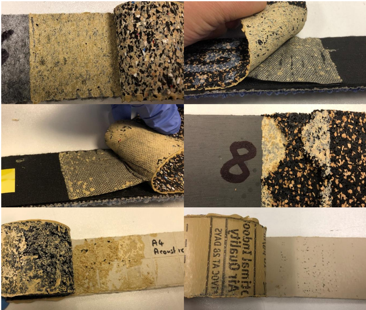
Figure 2 - Images of samples bonded using REGUPOL 46-101 adhesive after initial peel testing.
